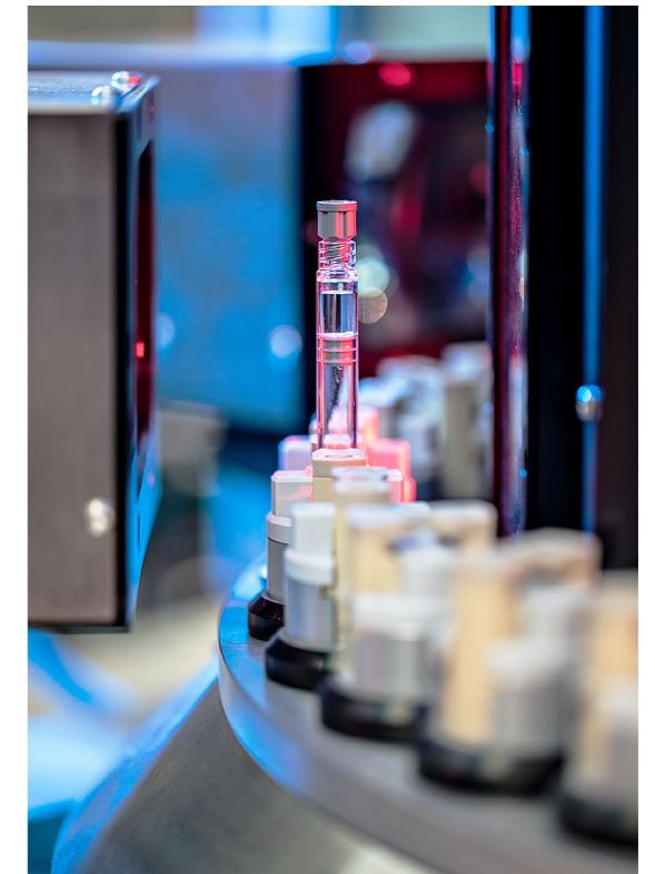
Air bubble or foreign body – Bubble-X knows what's floating in the lower part of the syringe.
